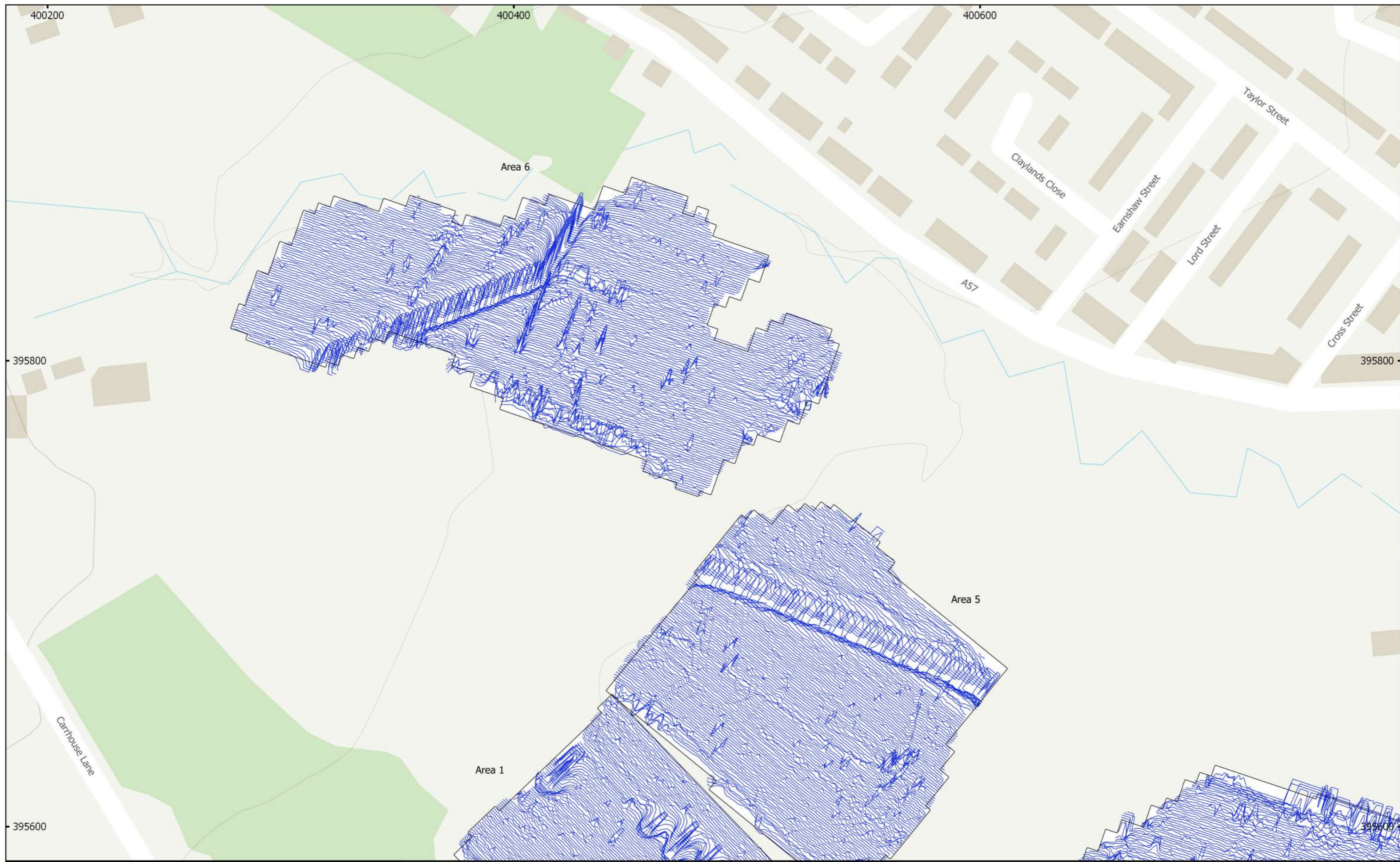
MSSK798B - Mottram, Greater Manchester Figure 10 - XY Trace Plot (Areas 1, 5 & 6) 30nT/cm at 1:1,500 @ A3 Copyright Magnitude Surveys Ltd 2021 Contains Ordnance Survey data © Crown Copyright and database right 2021
